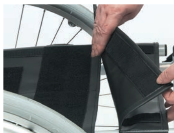
Decrease seat depth by 50mm for customised seat size.
