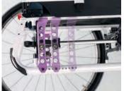
100mm centre of gravity adjustments can be made in 25mm increments which can even be fine-tuned to 12mm.
